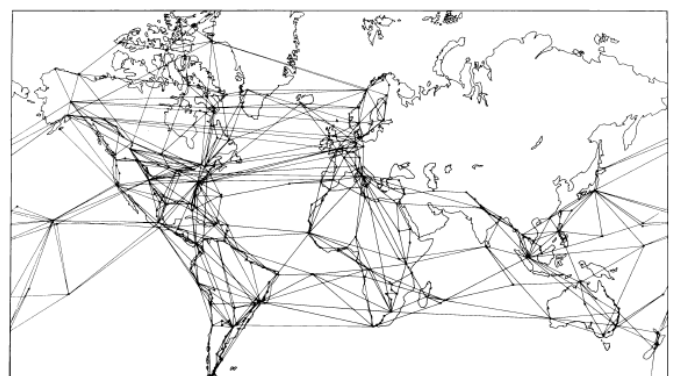
Fig. 4.1 : MAIN GRAVIMETER CONNECTIONS IN IGSN 71
