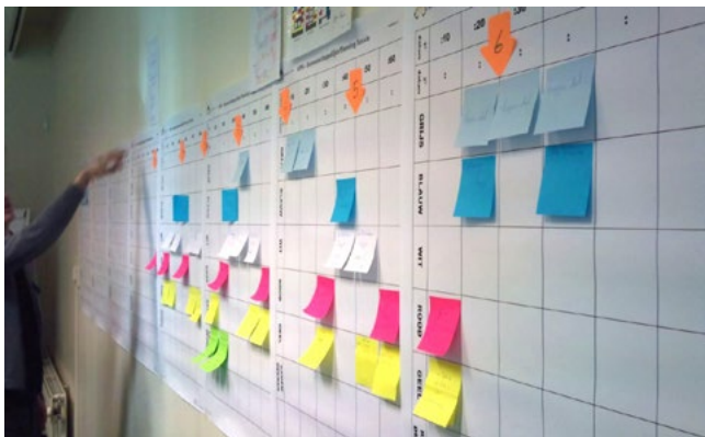
Slika 4: Vlečno planiranje (Pull Planning) na gradbišču (VIR: Lean Construction Blog, "Pull Planning in Design - Best Practices and Common Pitfalls")
